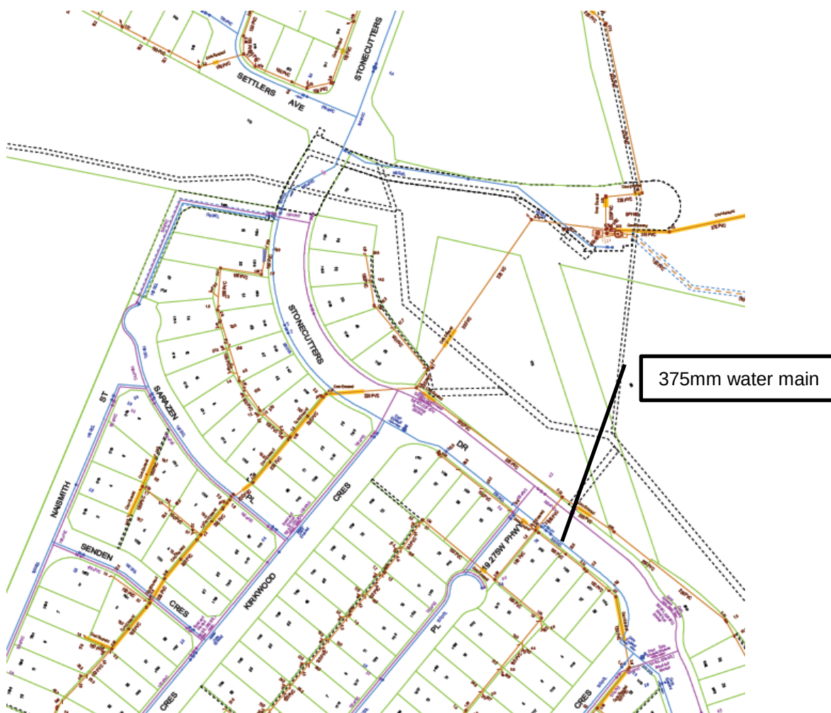
Figure 8 – 375mm diameter water main located in Stonecutters Ridge development
